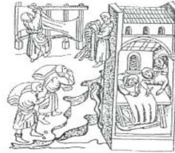
FIGURE 184—Cloth finishing in a monastery: (right) removing imperfections from the fabric; (left) stretching cloth on a tenter-frame. From an Italian manuscript of 1421.
