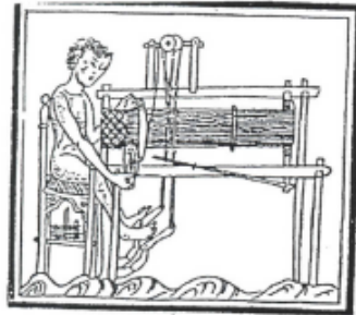
FIGURE 181—Horizontal loom with shedding-mechanism operated by treadles. From a thirteenth-century manuscript.
