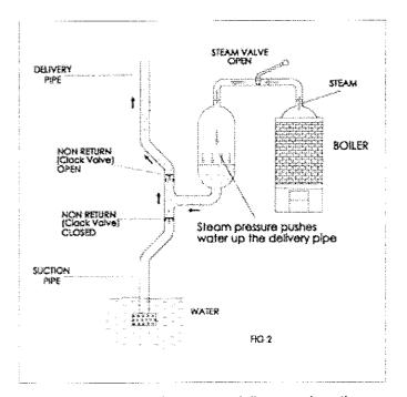
In practice, Savery's latest pumps had two vessels side by side, with common delivery and suction pipes. In this way he could have one pumping water out, whilst the other was filling with water ready to be pumped.
