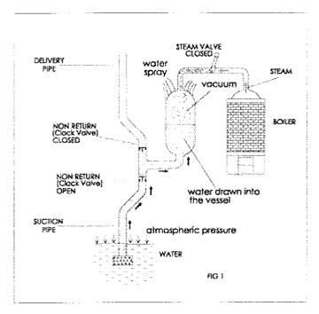
In FIG 1 the non return valve in the delivery pipe would be held closed by the weight of water above it. The steam valve was opened to fill the vessel with steam and then closed again. Water would be poured or sprayed on the outer surface of the vessel, which condensed the steam and caused a vacuum within. Atmospheric pressure would then push the water up the suction pipe to fill the vessel.
